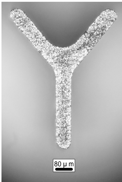
Figure 12. Dry EDM contouring sample
